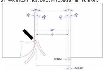
51" Wide Rolls must be overlapped a minimum of 5"
