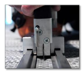
ii) <u>Cold welding</u> should not be done until the adhesive is completely dry. Protect the seam with masking tape at least 5 centimeters wide, pressing it down with a silicone roller to fix the paper tape well into the relief of the weave.
