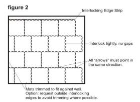
The interlocking tiles can be delivered with outside interlocking edge pieces at an additional cost if requested. The strips can be used to create a finished straight edge (See figure 2a).
