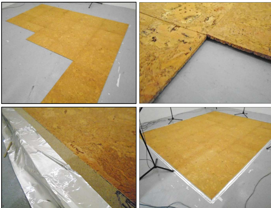
Images 4 to 7 Test specimen installation into the reverberation room
